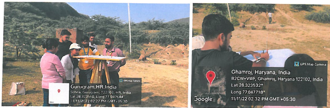
Photo 2 & 3: Students plotting the field dimensions using plane table survey method
