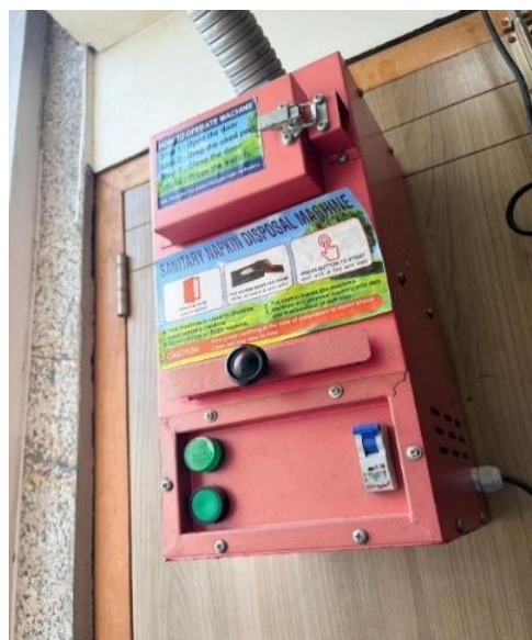
Sanitary Napkin Vending Machines and Incinerators installed in female washrooms to promote menstrual hygiene and sustainable waste management
